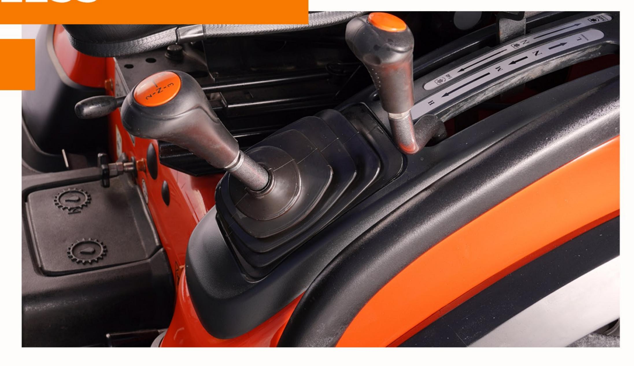
1<sup>st</sup> and reverse gears are in constant mesh with inline gear shift positions that helps in effortless & convenient shifting for operations involving front and rear movements like loader, dozer etc.
